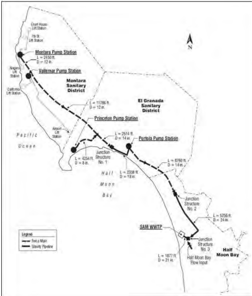
Figure 4. SAM Collection System Infrastructure
