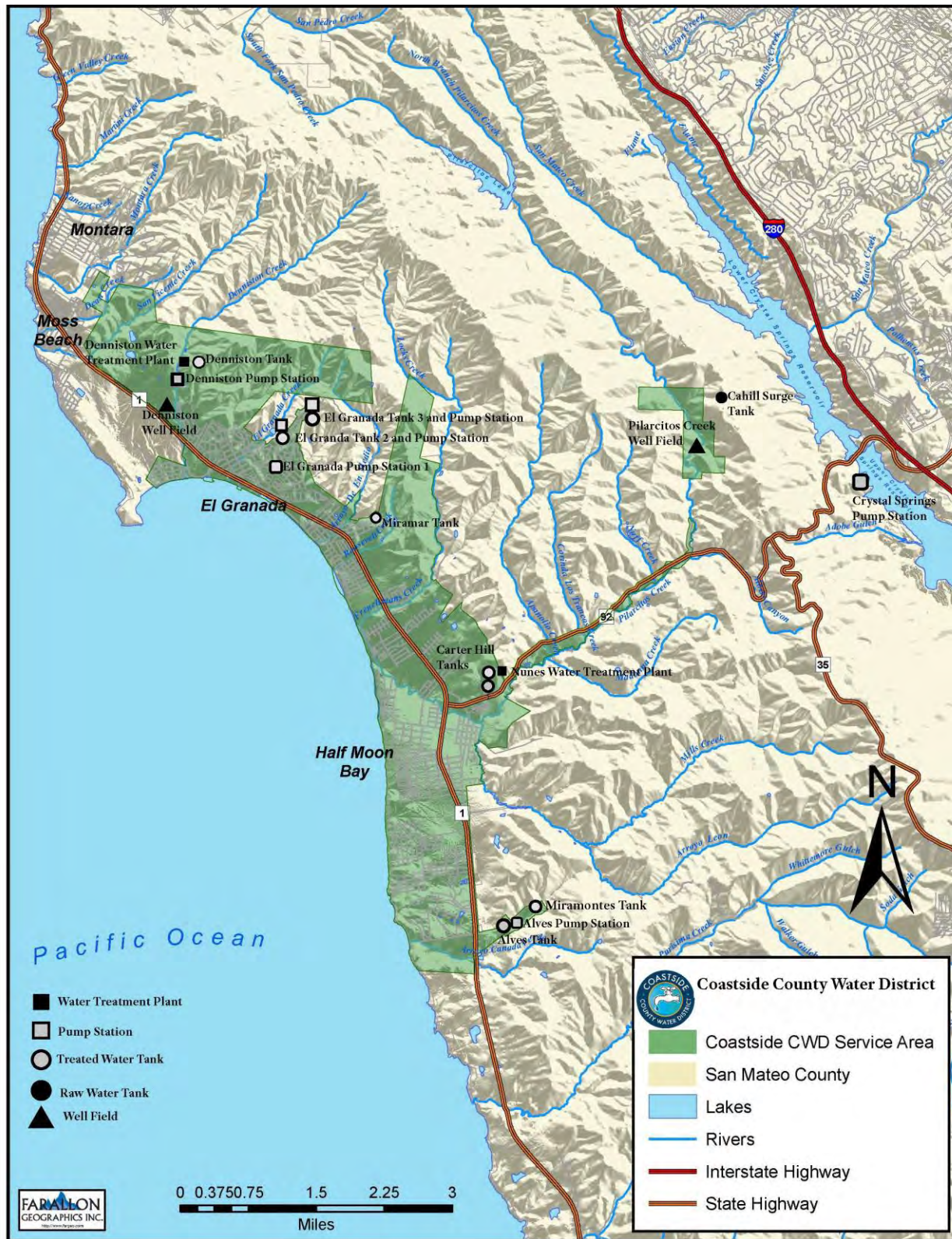
Figure 3-2. Coastside County Water District Water System Facilities
