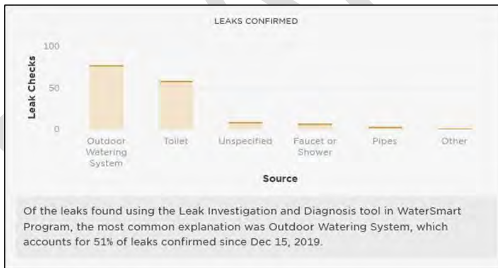
Figure 9-2. Source of Leaks Identified by the WaterSmart Program
