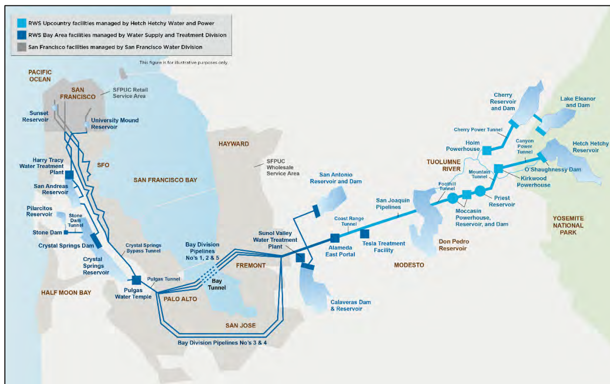
Figure 6-1. SFPUC Regional Water System and Main Facilities
