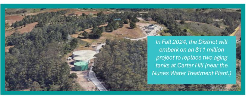
The Carter Hill Prestressed Concrete Tank and Seismic Upgrades project will involve the replacement of two steel tanks built in the 1950's with a 2.1 million gallon prestressed concrete tank. The new tank will require less maintenance and has an expected useful life of up to 100 years.
