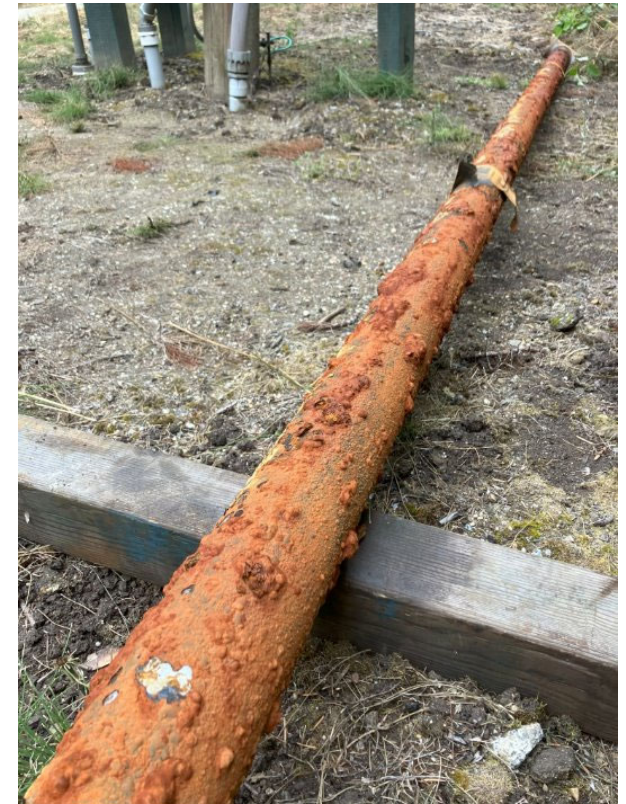
Scaling build up on existing pump drop pipe, which fouls well pumps and screens
