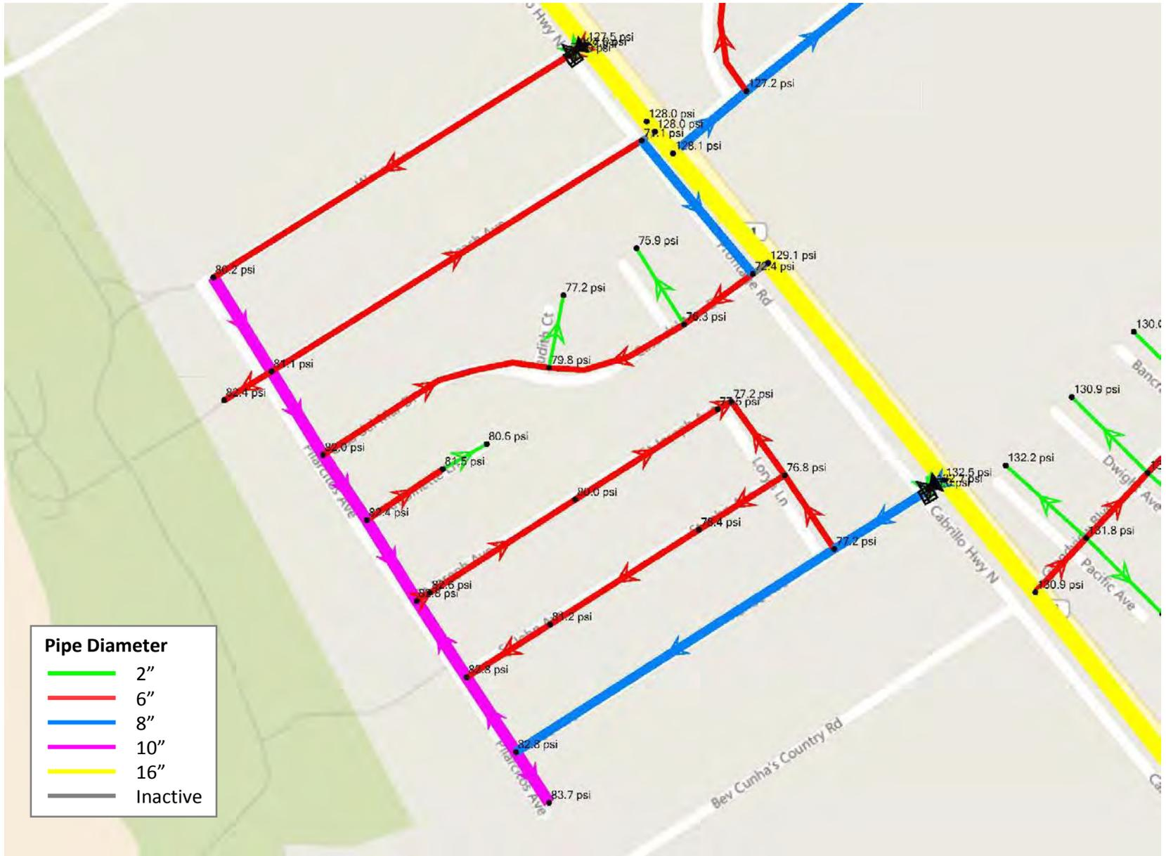
Figure B-1c. Modeled existing available fire flow in the Casa Del Mar area
