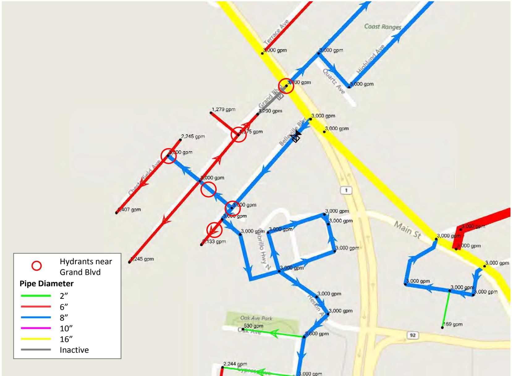
Figure B-2d. Modeled available fire flow in the Grand Boulevard area with proposed PRVs
