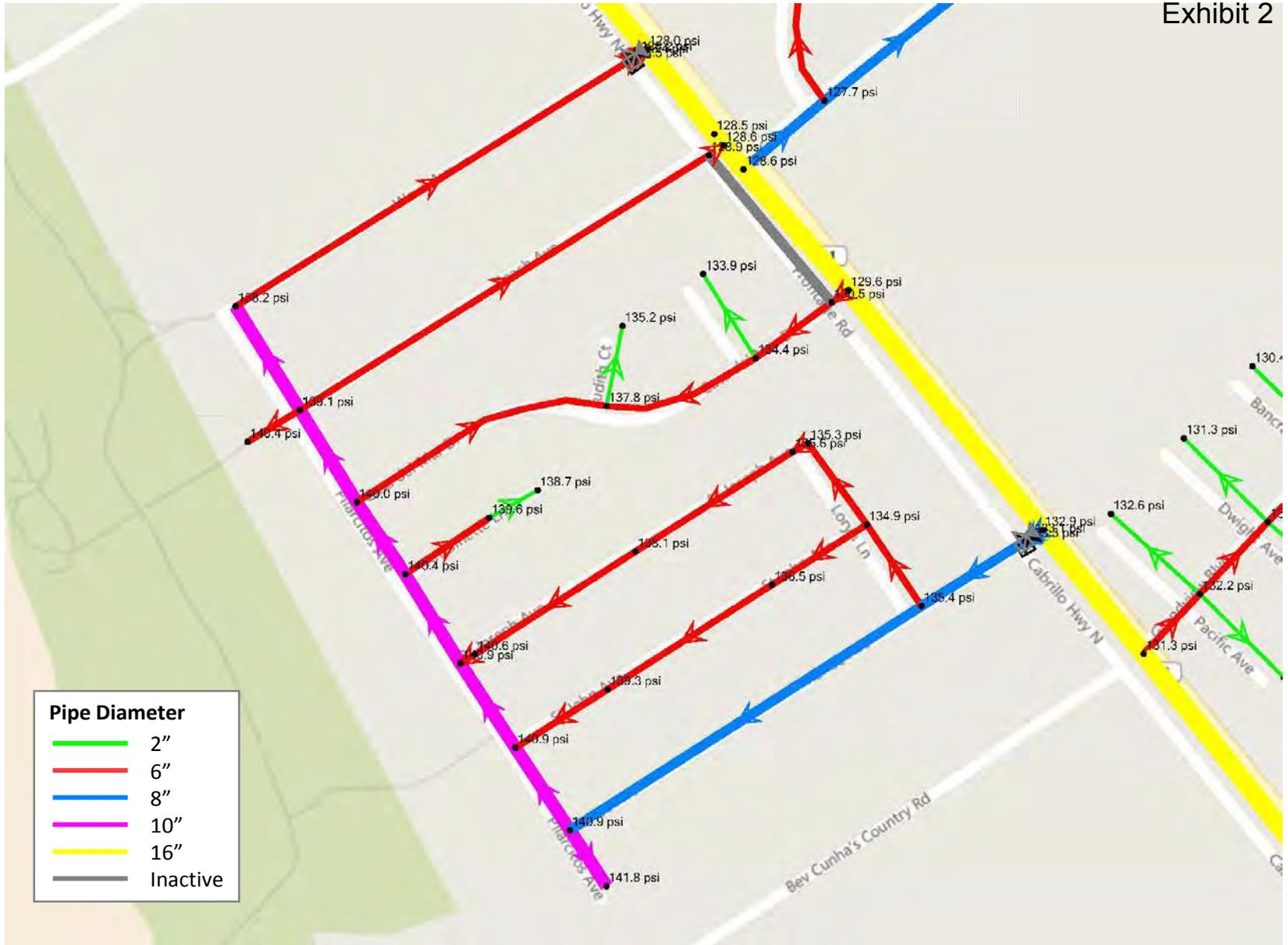
Figure B-1b. Modeled system pressure in the Casa Del Mar area with proposed PRVs
