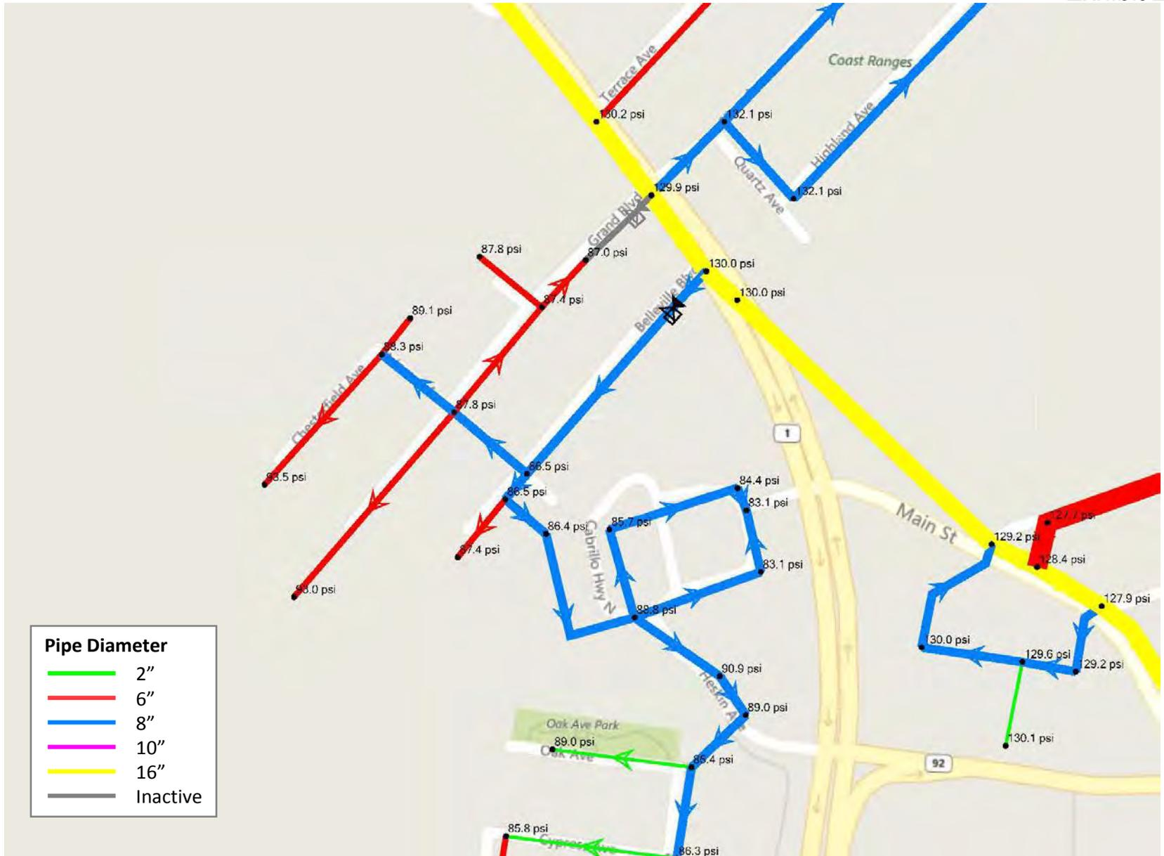
Figure B-2c. Modeled existing available fire flow in the Grand Boulevard area
