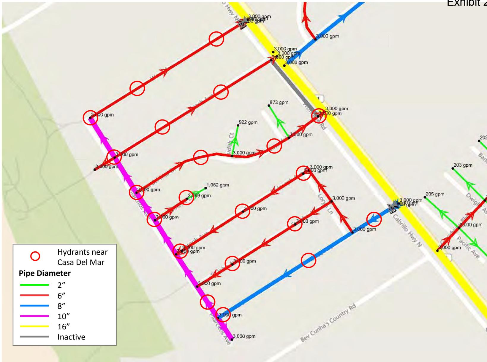
Figure B-2a. Modeled existing system pressure in the Grand Boulevard area
