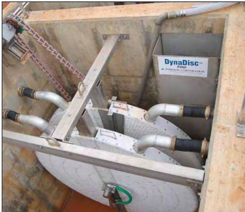
Figure 4.5 DynaDisc ® Cloth Media Filter
