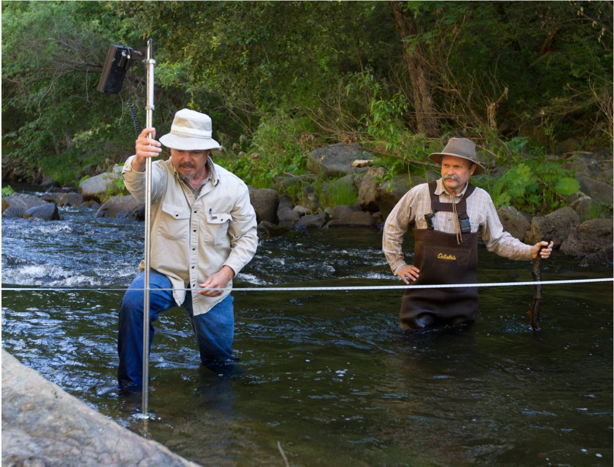
Dave Riffel and Hans Bayer (Hetch Hetchy Watershed Keepers) measure streamflow at the South Fork of the Tuolumne River.
