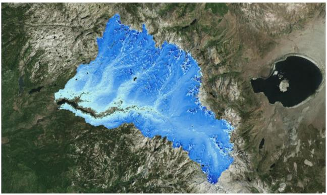
The Airborne Snow Observatory flew the Tuolumne Basin in February, providing us with the above map of snow depth through the Hetch Hetchy Watershed. Snow depths of up to 30 ft deep were measured in some high elevation canyons. At our Snow Survey sites, snow depths over 200 inches were measured. Nearly 1 million acre-feet of water is estimated to be currently stored as snow in the Hetch Hetchy Watershed.
