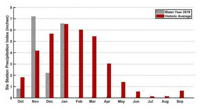
Figure 2: Monthly distribution of the six-station precipitation index as compared to the average monthly precipitation. The precipitation index is computed as the average of six Sierra precipitation stations and is an indicator of the overall basin wetness.
