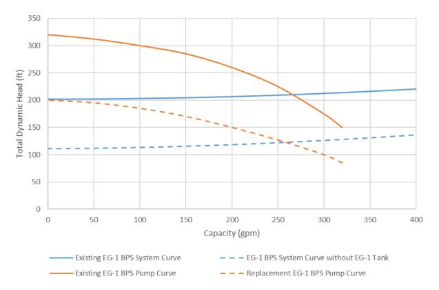
Figure 1. System Curve and Pump Curves at EG-1 Booster Pump Station (BPS) with and without EG-1 Tank
