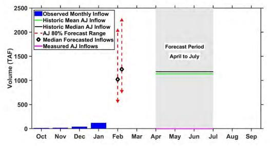
**Figure 6:** The Hetch Hetchy Water Supply Forecast Model (WSFM) was run before and after the early February storm. The current median forecast is above the long-term averages. All forecasts have sufficient inflows to refill the Tuolumne River System by the end of runoff.
