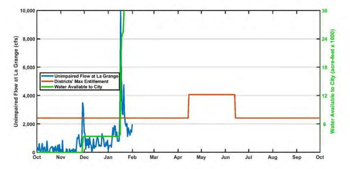
Figure 5: Calculated unimpaired flow at La Grange and the allocation of flows between the Districts and the City. To date there has been over 78,000 ac-ft available to the city in Water Year 2019.
