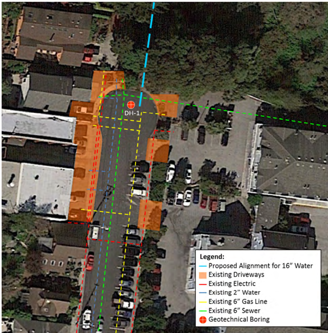
Figure 3 – Trenchless Crossing Site South of Pilarcitos Creek
