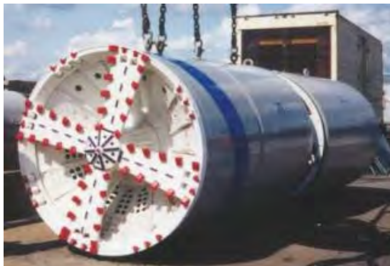
Figure 5 – 72-inch Akkerman Microtunneling Machine (MTBM)
